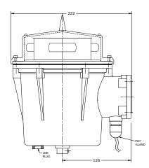
Light-Head with integrated power supply • Omni directional low intensity light ( 2000 cd). • 4 optics with cover in hard polycarbonate and Powder-coated aluminum enclosure
